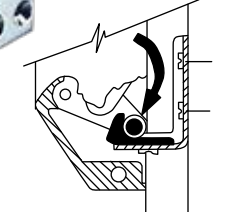
POSITIVE PRESSURE SEAL CROSS SECTION DETAIL
